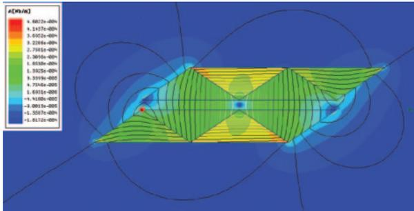
▲ Magnetic field emitted by one-sided structure under zero shear condition. The triangles are magnetic blocks, and the rest of the image is air. The highest field intensity is orange, and the lowest is dark blue. The lines that travel across the gap illustrate attractive forces.
