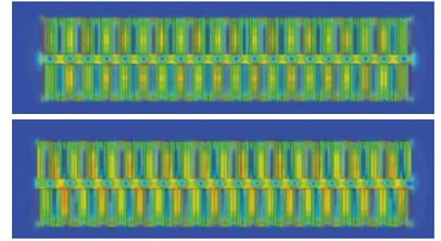
▲ Two continuously varying substrates aligned have a large attractive force (top). The pattern in the upper magnet has been shifted to the side and illustrates a maximum shear force condition (bottom).
