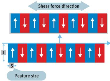
▲ Alternating blocks of magnetic material are used to produce magnetic shear forces.
