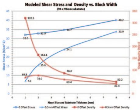
▲ The effect of block width on measured shear stress and density
