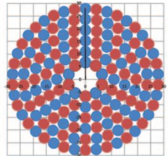
▲ Pattern of tracks printed on magnet to produce high-performance magnetic clutch
