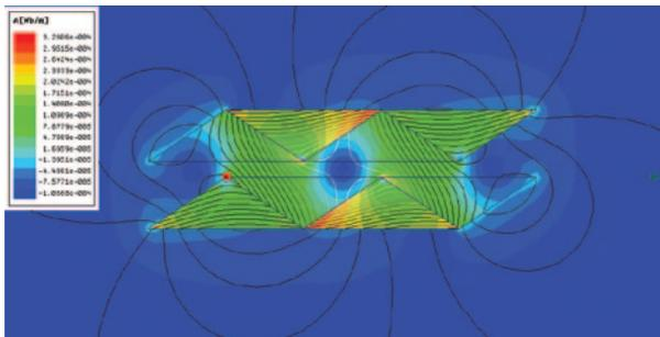
▲ Magnetic field emitted by one-sided structure in a maximum-shear condition. The highest field intensity is orange, and the lowest is dark blue. The lines that travel across the gap illustrate attractive forces.
