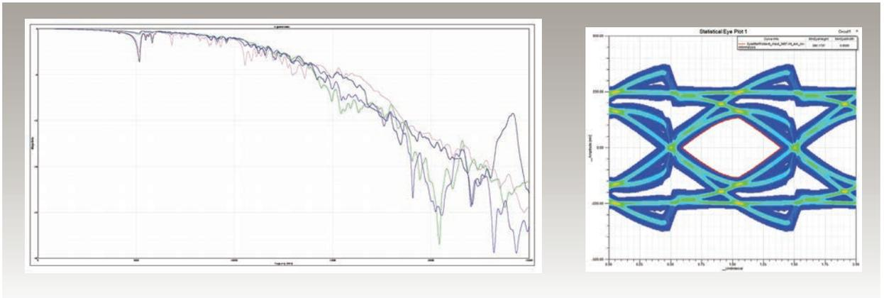
▲ An example of notch behavior and resulting eye diagram that shows margin
