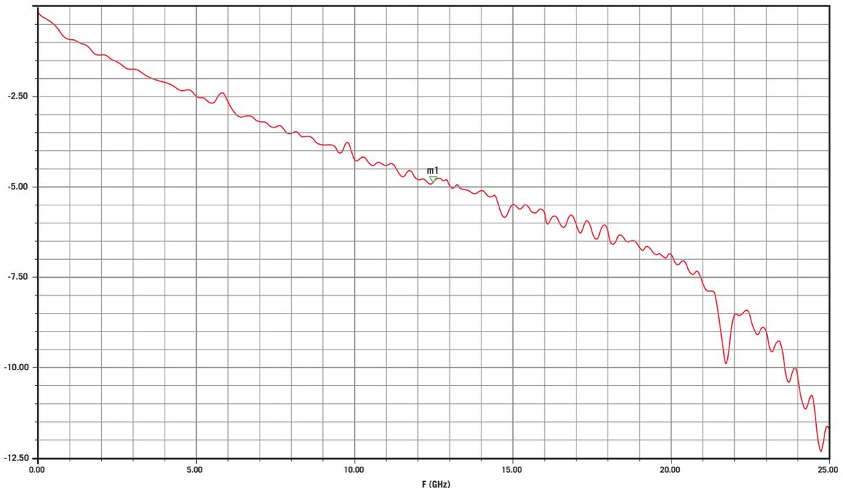
▲ ANSYS HFSS S21 insertion loss plot of the extracted channel
