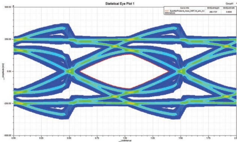
▲ Statistical eye diagram plot of the 28 Gb interface shown in the circuit simulator
